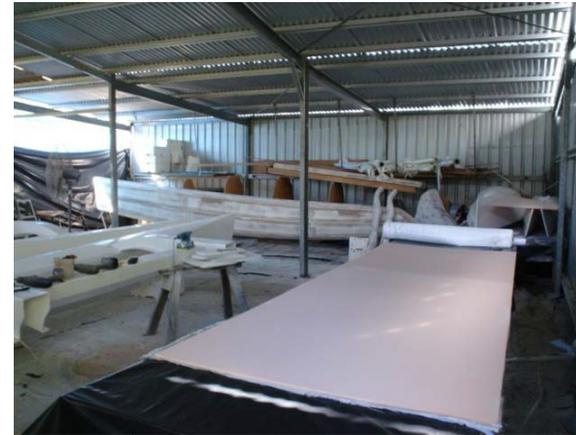
To loft the boat panels a straight line is drawn on the edge of the fabricated panel and the line is marked at 500mm intervals. A square can be used to draw lines perpendicular to the base line. Mark the dimensions given on the plans along the perpendicular lines. Panel pins are nailed at the marks and a flexible baton is bent to create a smooth line. The baton can be made from a narrow piece of plywood the length of the overall panel. Draw the lines onto the peel ply.
